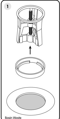
**1.** The first step is to find which Ring suits your basin waste. We recommend you try the Black Ring first and then work down to blue and then green. This will reduce the risk of dropping the Expanding Insert down the waste.
