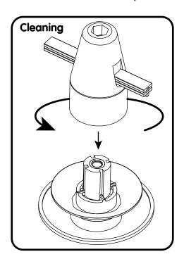
**Cleaning.** We advise that you clean your plug regularly to avoid any substance obstructing the waste. To do this simply unscrew the plug and clean any debris.
