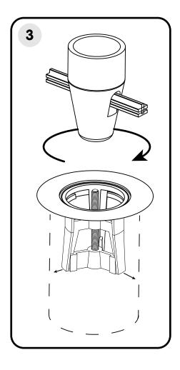
**4.** Fully screw the Converta Plug onto the Expanding Insert. Click the plug a few times to test if the spring is working. Then fill up your basin and test if the plug is working effectively.
